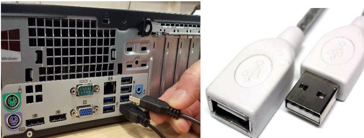
Fig 1. Connecting the keyboard and mouse to PC via the USB slots
